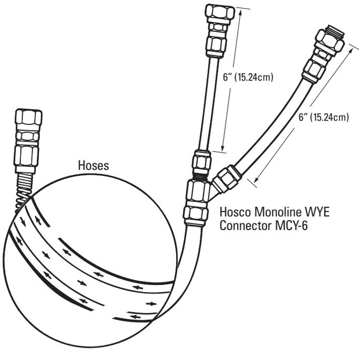
Hosco MCPHA (Monoline Coaxial Paint Hose Assembly) is a unique and novel method of circulating paint or any fluid with the appearance of a single hose system. This innovation reduces the hose management issues at dispense or spray stations for materials needing recirculation by supplying the material in the annulus area between the outside and inside hoses, and returning the material being circulated thru the inside hose ID.
