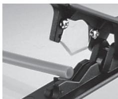
The Hosco Hose & Tubing Cutter will provide straight, clean, accurate cuts for optimum fitting connections. The lightweight, rugged unit will cut 1/8" through 3/4" OD tubing. The exclusive "blade guard" feature provides protection from accidental blade contact. Ribbed handle aides in accurate positioning on the tube.
