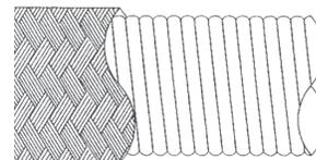
PSHC – conductive (carbon impregnated), PTFE lined, fiberglass reinforced innercore, overbraided with 300 series stainless steel.
