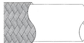
PDHC – .030 wall, conductive lined, virgin PTFE tubing, overbraided with 300 series stainless steel wire.
