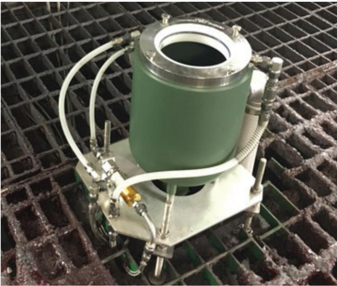
Shroud cleaners in any coating application can be a primary source of “dirt” and surface defects if not properly and continuously maintained, which stems from increasing production and manpower demands.
